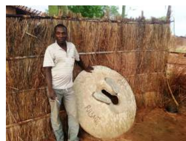
Figure 1: Artisan and concrete latrine slab in the town of Ribáuè.
