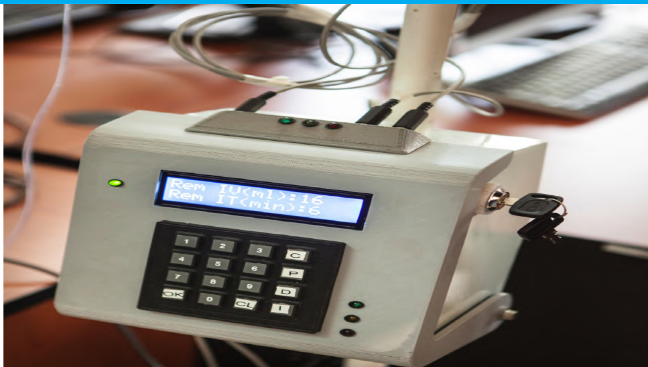
An Electronically Controlled Gravity Feed Infusion (ECFG), a new technology that controls the rate of fluid flow administered to patients.
