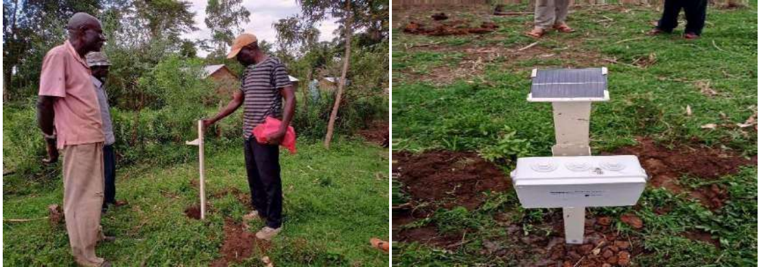
Figure 6: Deployed prototype of the mini-weather station
