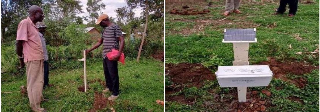
Figure 6: Deployed prototype of the mini-weather station
