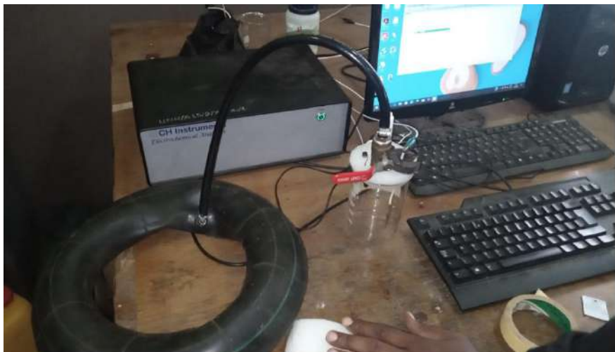
Figure 2. Setup for corrosion test using the electrochemical workstation.
