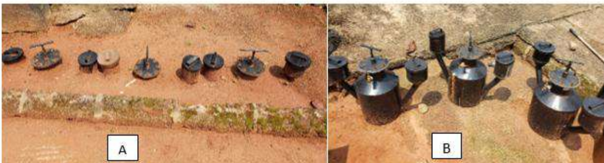
Fig.1. Experimental Set Up of Fixed Dome Biogas Digesters (A)Buried Underground (B) kept on the surface uninsulated
