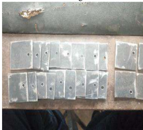
Figure 1. Steel coupons for corrosion test.
