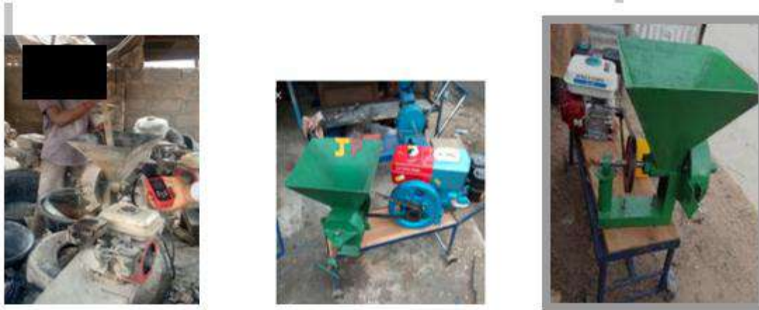
Fig. 2(a) Cassava milling machine (b) Bambara nut milling machine (c) Tomato grinding machine
